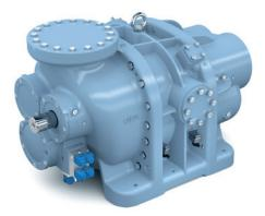
The GEA Grasso LT series comes in fourteen sizes and covers a swept volume from 805 to 8560 m<sup>3</sup>/h. Due to the combined sleeve and roller bearing of the rotors, the compressor has an extremely long life span and low noise and vibration levels. All components are designed for long operating life, high availability and easy maintenance. Furthermore, the compressors of the GEA Grasso LT can be provided according to the API 619 standard and ISO 10440, respectively.
